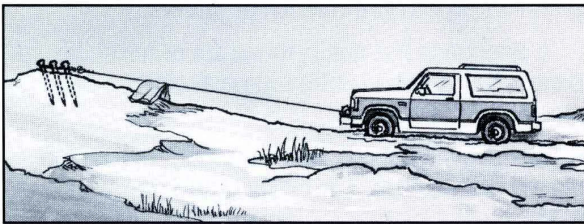
Stakes driven in solid earth and chained together make a good anchor point for self recovery when no solid anchor point is available.
